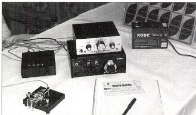
Keen QRP operator Clemed Nilsson SM7DRM's station showing solar panel power supply (see text).
